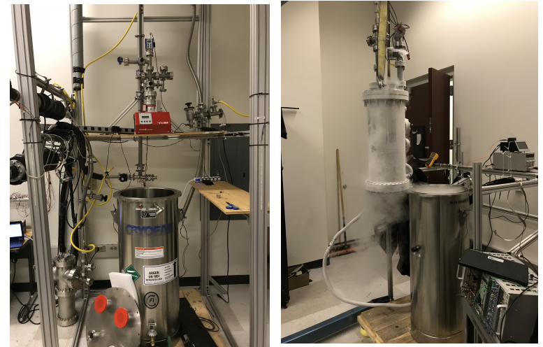
Purification System as built at UTA with the smaller 117 liter cryostat
