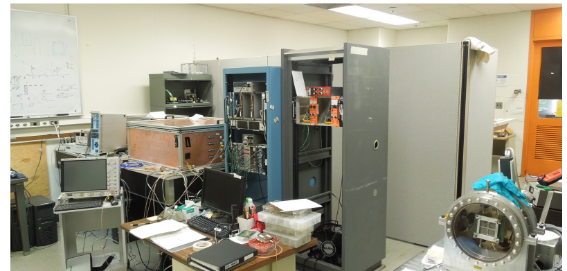
Photomultiplier Lab – characterization and testing: diode laser integrated in dark box, vacuum test chamber
