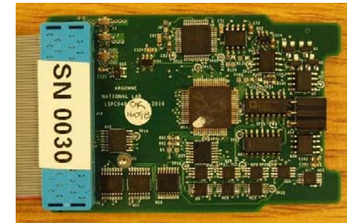
Front End Electronics Reside inside Base
