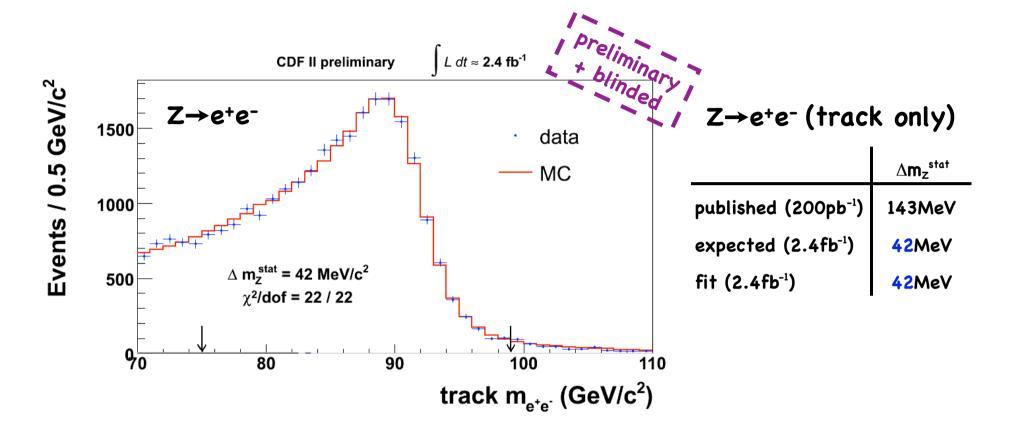
Sensitive to photon emission modelling (bremsstrahlung).
