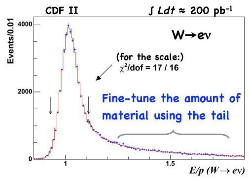
Non-linear calorimeter response also simulated (measured on E/p)
