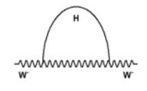
Radiative corrections ( $\Delta r$ ) dominated by top quark and Higgs loop allows constraint on Higgs mass
