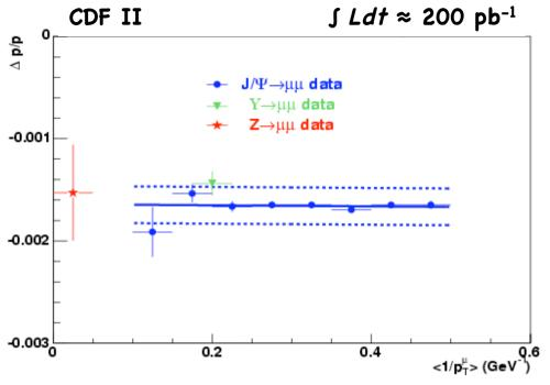
A combined  $J/\psi$  and Y(15) momentum scale, with the cross-check in  $Z-\mu\mu$
