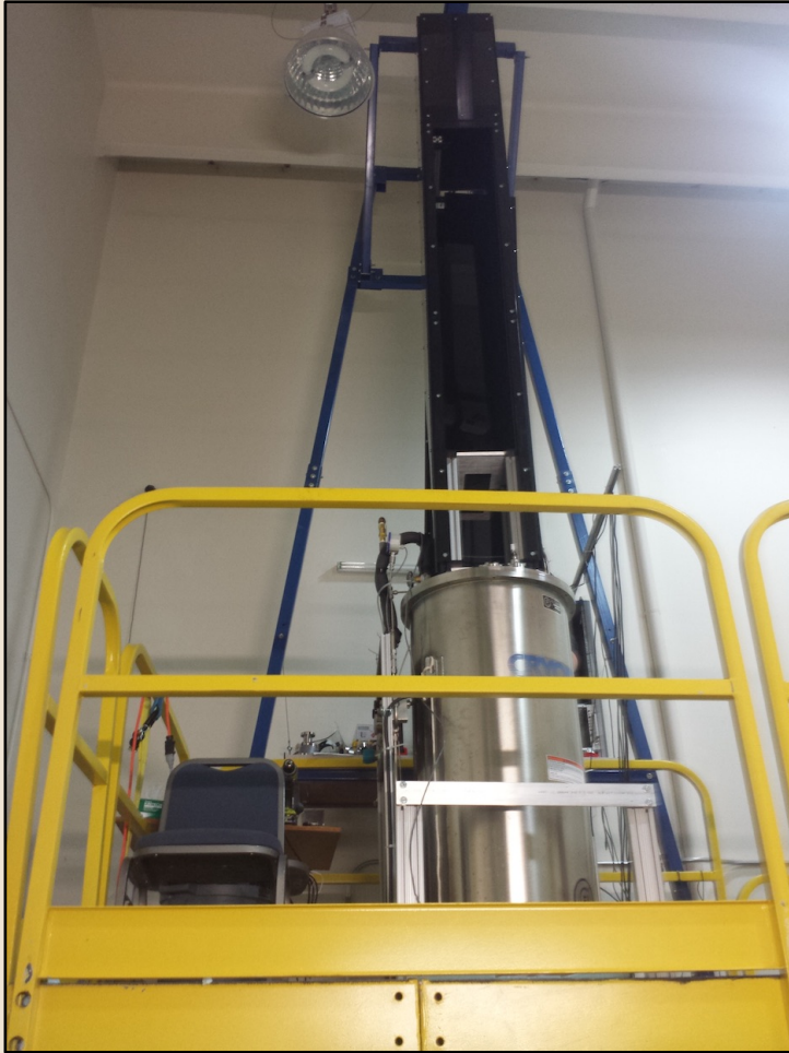
Mechanical test apparatus for mechanical tests of up to 4 PDs in LN2 (500 l dewar at CSU)
