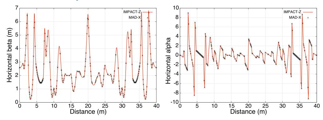
Space charge off, sextupoles off, no RF Zero energy spread, zero bunch length (transverse dynamics only)
