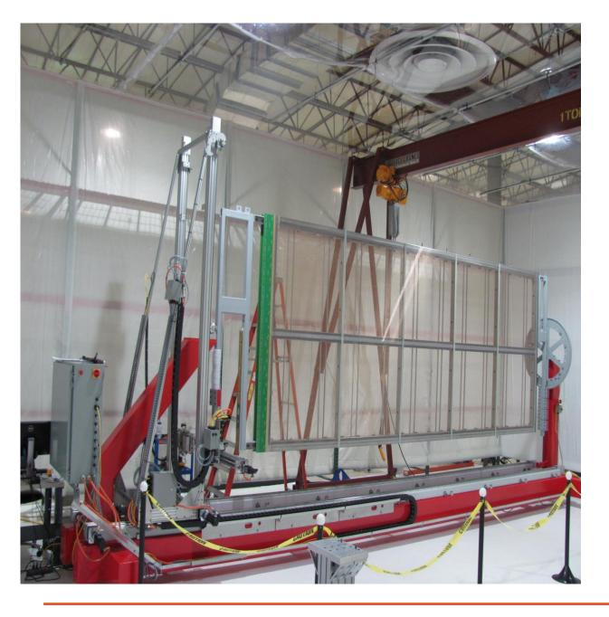
Full scale ProtoDUNE APA in the winder. The fundamental difference between these APAs and those planned for the far detector is the thickness of the frame material and the addition of conduits for routing CE cables.
