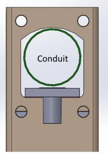
The link has been planned in G10 – and calculations show good safety margin. However, we are going to consider making it stainless steel for increased strength, with with G10 linings to insulate it from the frame.
