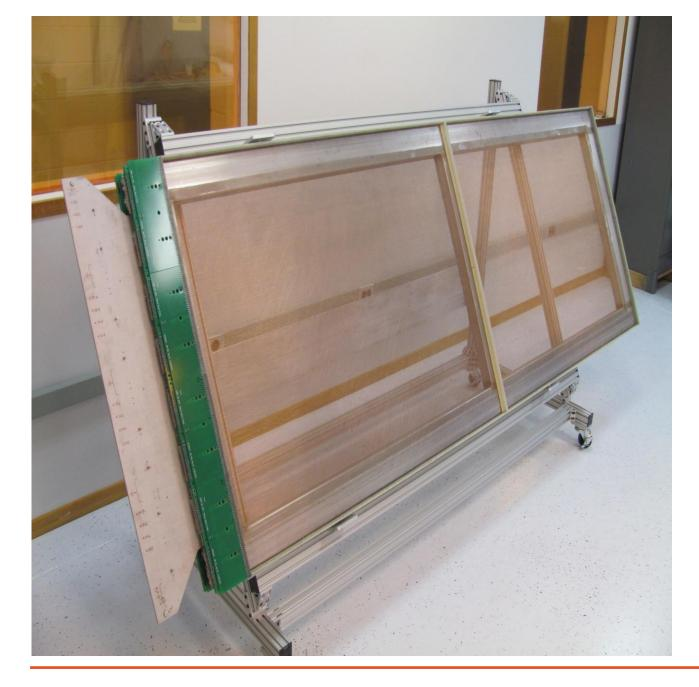
40 percent scale APA built at PSL. The concept originated with Bo Yu. It was a continuously wound concept – winding was done essentially by hand. The U and V plane wire angle was 45 degrees at that time.
