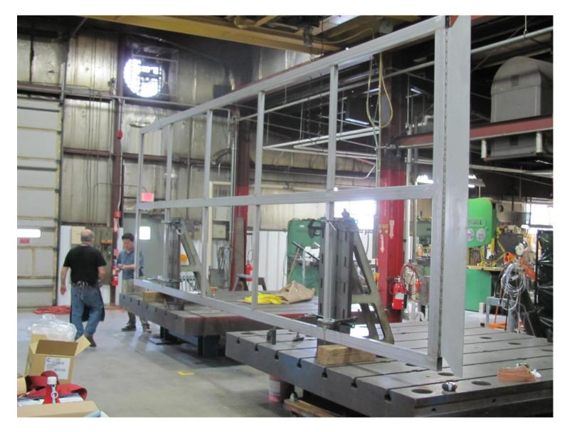
A 7m x 2.5m frame was built in 2013. This frame was a monolithic weldment. It was time consuming to build and flatness was difficult to achieve. Note the fin at the head.
