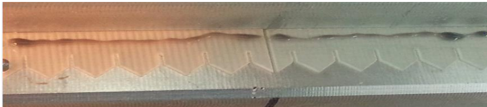
A thin line of properly dispensed 2216 G epoxy is seen near the flat edge of the comb.
