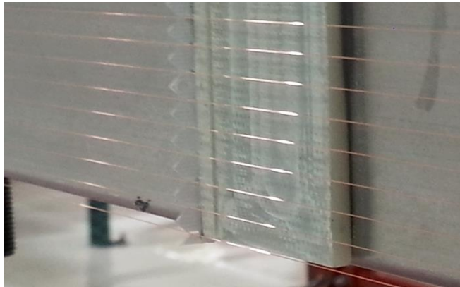
Wires routed through a comb base of the X-plane and wound wires laying across one of the X-Head board solder pad areas.
