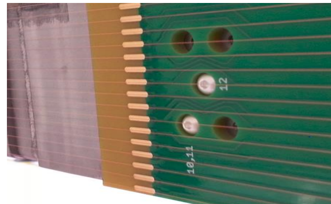
Wires routed through a comb base of the X-plane and wound wires laying across one of the X-Head board solder pad areas.
