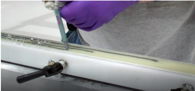
Applying (3) stripes of 2216 Gray Epoxy along the cleaned bottom of the Comb Base Assembly while loaded in the installation jig.
