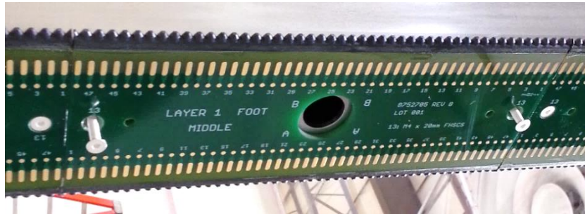
Middle X – Foot Board Assembly attached w/ (2) M4 x 20mm FHSCS
