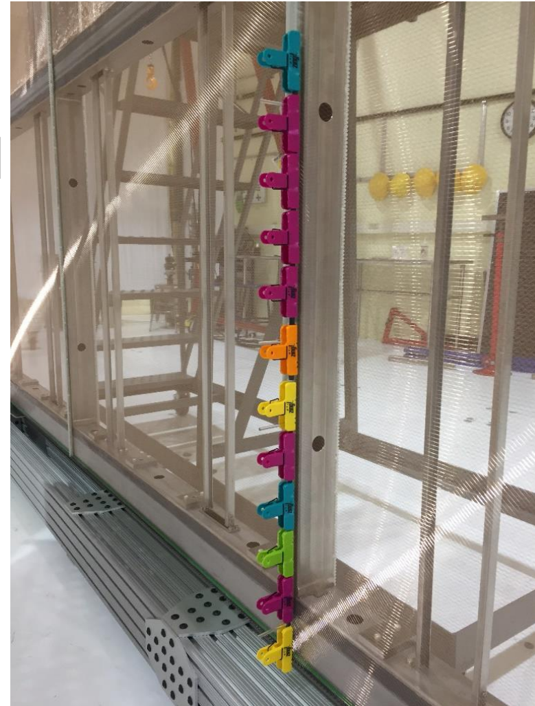
'V' Combs clamped in position for adhesive cure time
