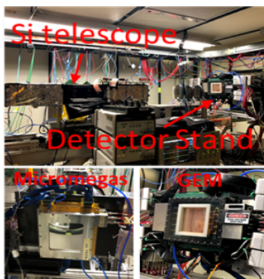
Figure 32: Detector setup in beamline, including use of FTBF Si telescope
