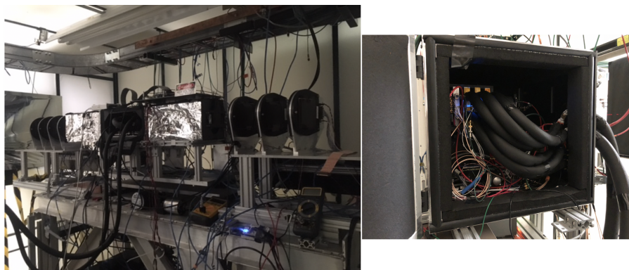
Figure 29: A picture of the experimental area. The pixel telescope detectors are placed inside the electrostatic-discharge shielded boxes on the two sides of the DUT area. Cold box with mounting frames for LGAD sensors is shown on the right.
