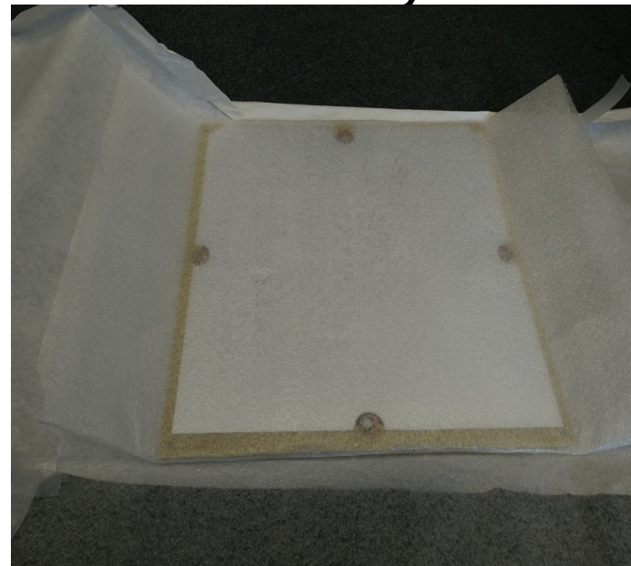
CPA plate with Glued on Reflective foil.
