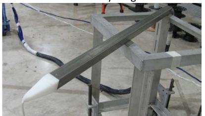
The first ~1.4m cable bundle – where the connectors are, is covered. It's a 2" x 2" tube with a nosepiece to help guide it through the openings.
