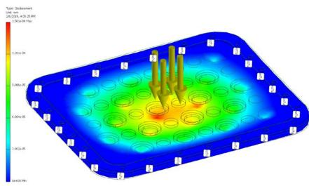
1 psi from outside cryostat:  $^{\sim}0.2\mu m$ displacement
