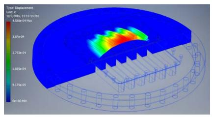
1 psi from outside cryostat: ~12μm
