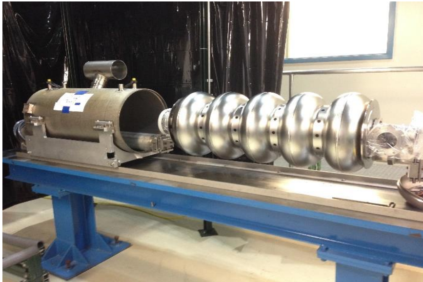
Cavity dressing mock-up
