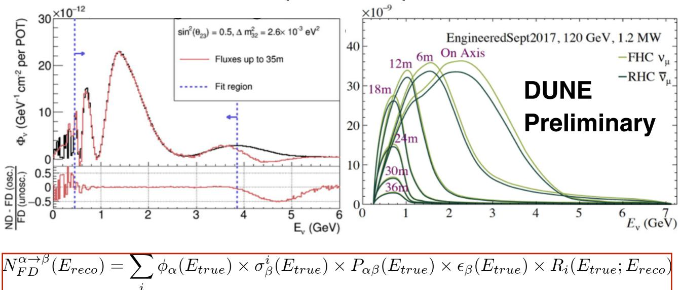
Many near detectors can approximate far detector oscillated flux! Changing beam line optics can help, too.
