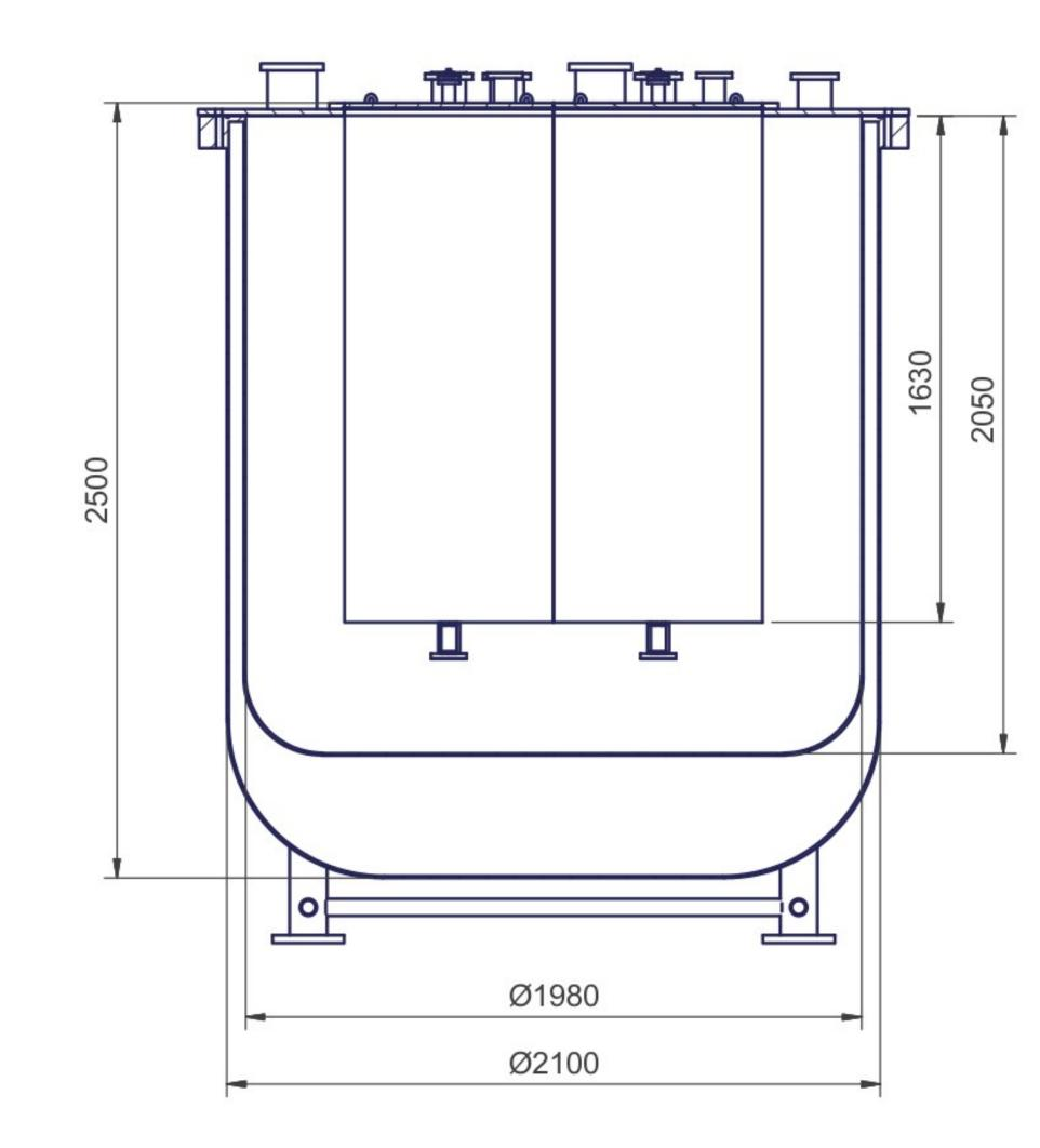
Vacuum insulated & LN2 cooled cryostat. 8.6 t total LAr. 1.7 t active LAr.
