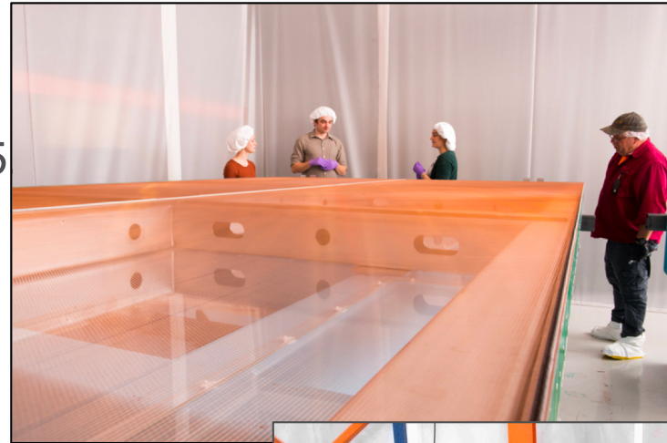
1 st UK APA on the alignment fixture
