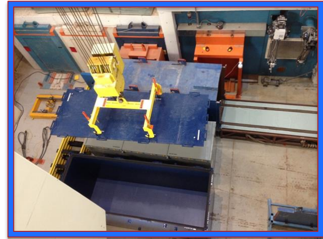
Lowering of 7A Lid for IP-1 Closure
