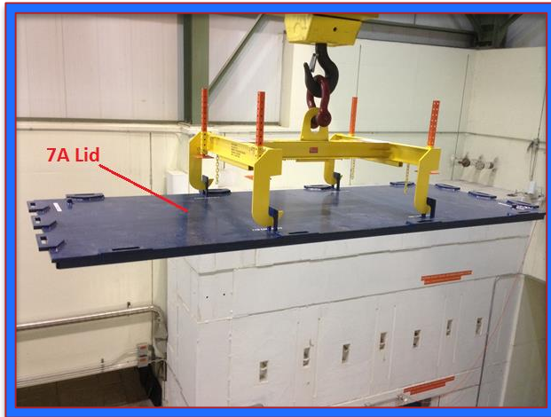
Fixture Attachment to 7A Lid
