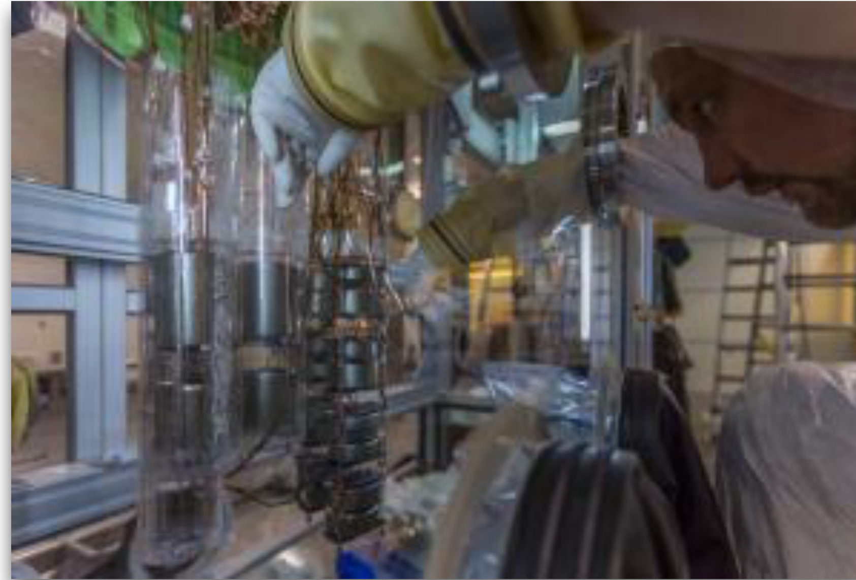
Building the GERDA detector array in the glovebox © J. Suvorov, GERDA collaboration
