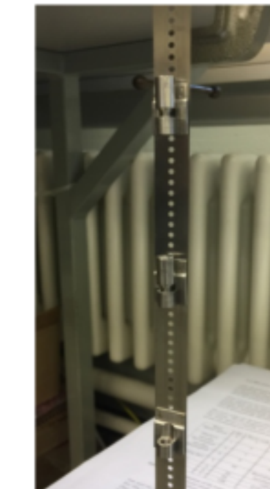
Spot-welded source holders
