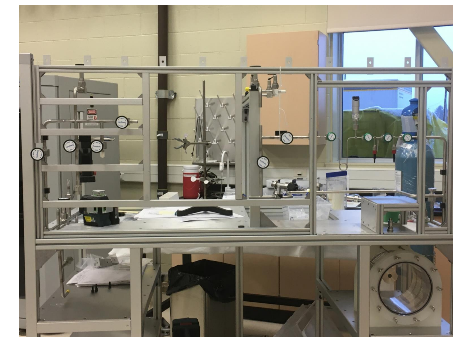
One of SNOLAB's radon emanation chambers and cold-traps.
