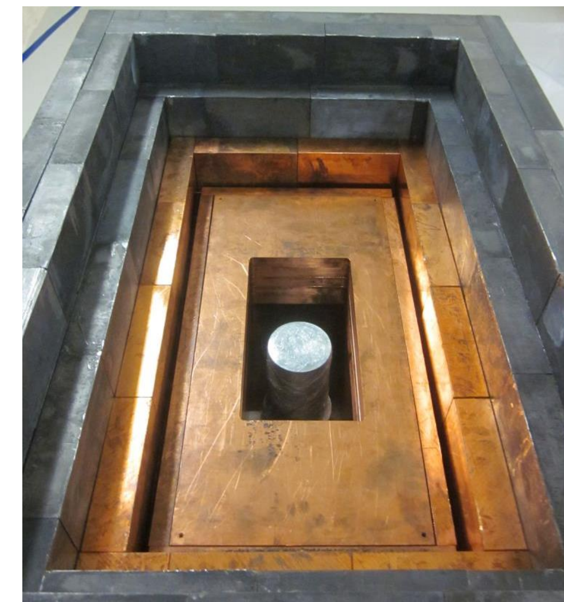
One of the High Purity Germanium Counters along with its copper and lead shielding.
