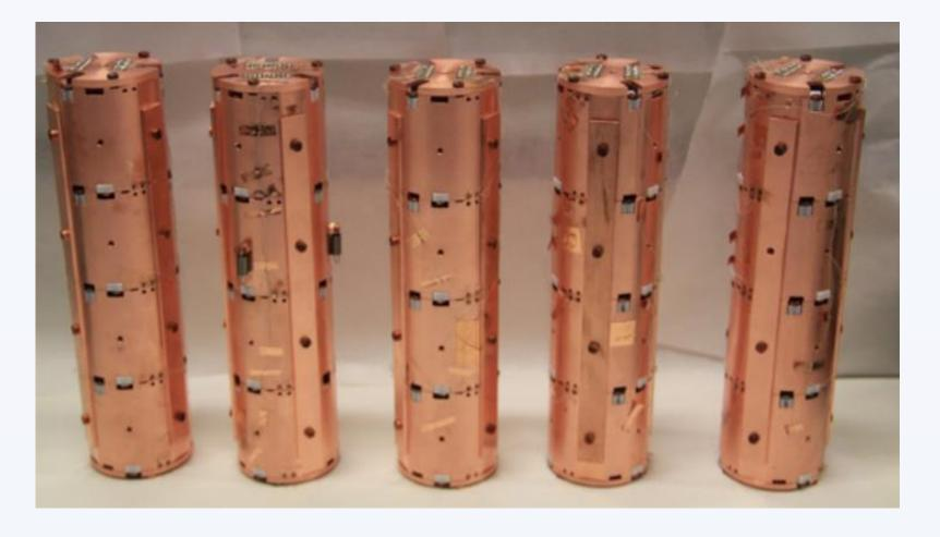
The detectors exhibit extremely high energy resolution (FWHM~6 keV for 2615 keV gammaquanta) investigated with Th/U sources. However, a dirrect measurement of the energy resolution at Q-value of <sup>100</sup>Mo (3034 keV) is impossible with a Th/U source. It is crucial to cross check the calibration and the energy resolution by means of sources providing gamma peaks at energies higher than the range of interest of <sup>100</sup>Mo.
