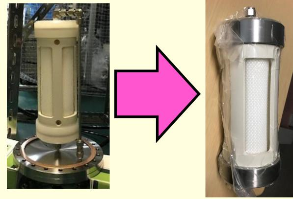
Now, new membrane module has being developed which has SUS cap. The radon emanation from the new membrane module will start.
