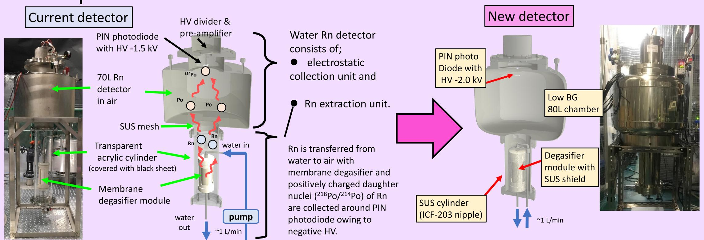
70L Rn detector has higher BG mainly due to rubber sealing and corner shape of chamber > Lower BG 80L Rn detector [2] Acrylic housing for membrane is also sealed with rubber O-ring  $\rightarrow$  Replaced with stainless steel (SUS) housing.
