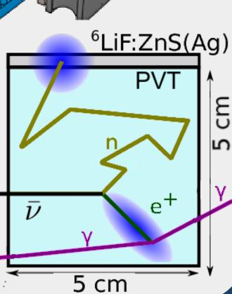
Light, generated in a scintillator cube and sheet, is guided by a grid of fibers to sensors. With 12800 cubes and 3200 fibers and sensors, energy calibration does not come easy.
