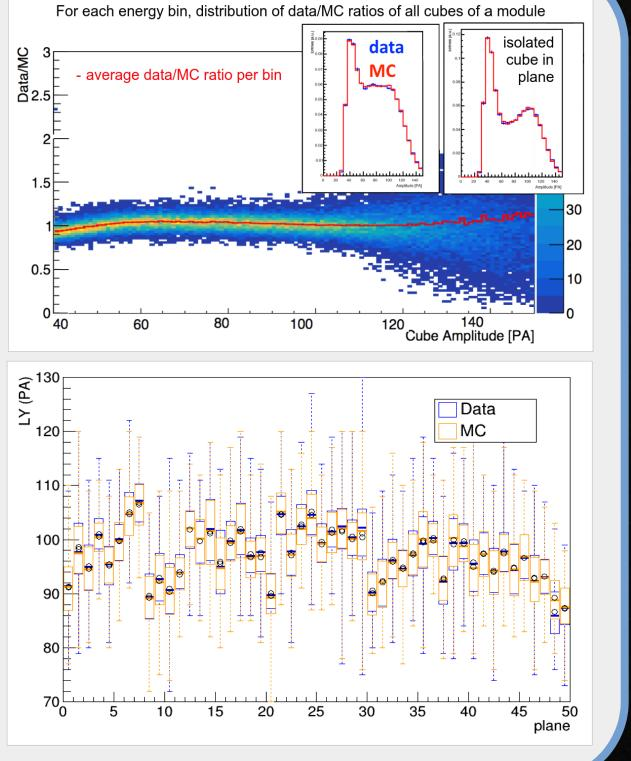
• Calibration and simulation of SoLid detector energy response are crucial to correct detector inhomogeneities and perform a precise neutrino oscillation measurement
