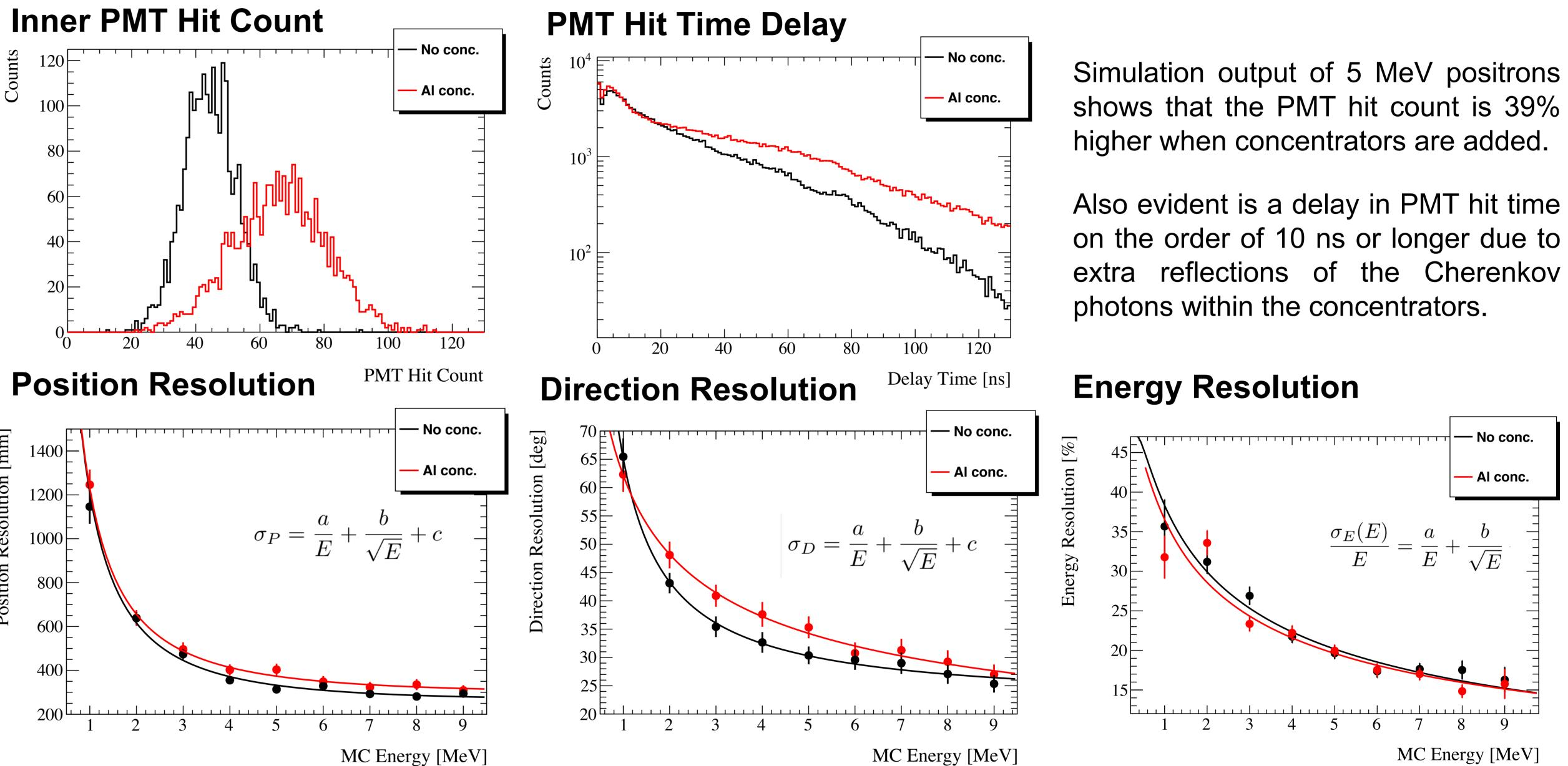
The position, direction, and energy resolution of simulated 0-10 MeV positrons was fitted to the standard formulas. Due to the delayed effect concentrators have on PMT hit time, reconstruction deteriorates slightly. This results in slightly worse position and direction resolution when concentrators are used. However, the significant increase in collected light improves energy resolution.
