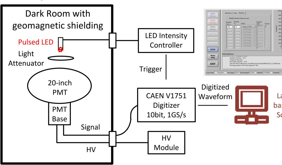
PMT output waveforms were captured and digitized by a 10-bit fast ADC. The record window is 21 µs after the LED trigger, covering the **measurements on the** baseline, main pulse and the afterpulses. Waveforms of the dark counts were measured with LED off and the same condition as the afterpulse measurements.
