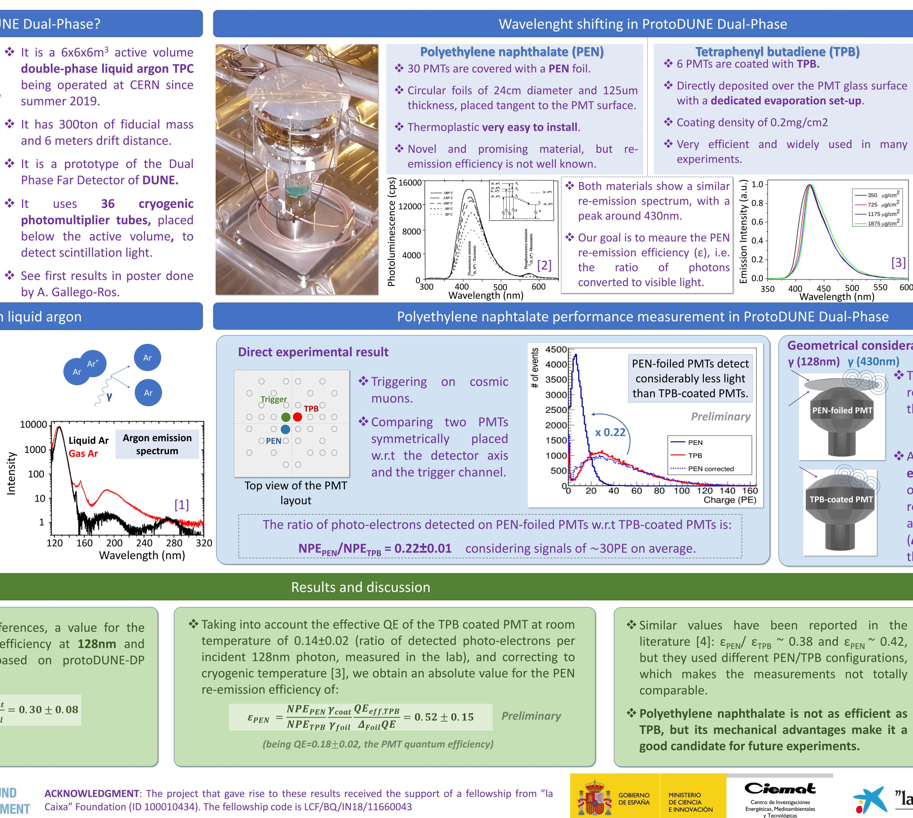
Correcting the geometrical differences, a value for the relative PEN/TPB re-emission efficiency at **128nm** and 87K/cryogenic temperature based on protoDUNE-DP measurements is obtained: Preliminary
