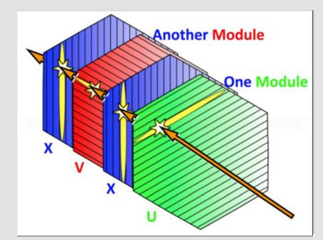
X, U (+ 60°), and V (-60°) oriented planes designed for 3D tracking!
