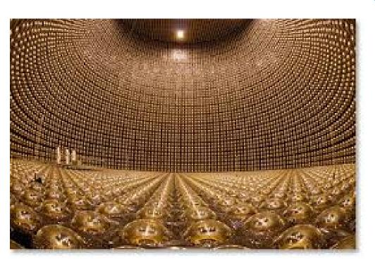
SK's inner detector contains 11146 photomultipliers (PMTs) with 3 ns time resolution. A typical event in SK lasts at most 200 ns. SK has gone through four phases of running. This analysis focuses on phase IV (2790 days).
