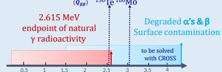
CUPID (CUORE Upgrade with Particle IDentification) adopts a method to reject surface  $\alpha$  events in bolometers exploiting the scintillation ( $\text{Li}_2\text{MoO}_4$ ) or Cherenkov radiation ( $\text{TeO}_2$ ) emitted by the absorber, since  $\alpha$  &  $\beta$  have different light yield.
