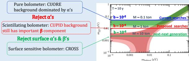
CROSS proposes a technique to mitigate surface contamination via providing bolometers with surface sensitivity → no light detector is needed
