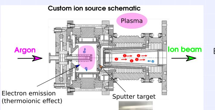
Extraction potential 20-50 kV ~10 nm of implantation depth
