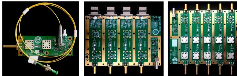
Fig. 2: Left: The front-end amplifier and RFoF transmitter. Center: The down-hole RFoF receiver and amplifier. Right: Surface amplifiers.
