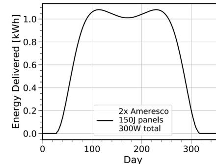
Fig 5. Expected delivered power from solar panels.
