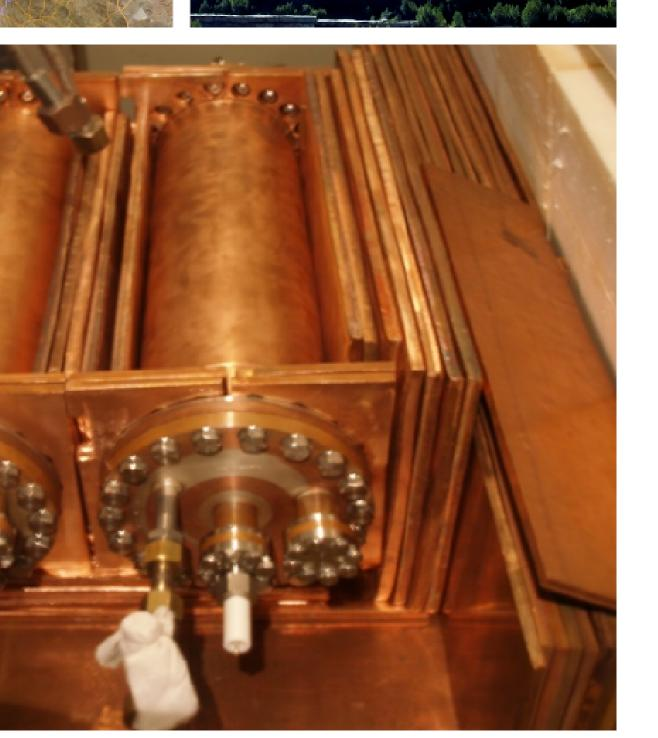
The experimental setup was located in the lowbackground laboratory of Baksan underground facility (4900 m. w. e). The large gas proportional counter consisted of copper cylinder  $(l = 735 \text{ mm}, \varnothing = 137 - 150 \text{ mm})$  and was filled with 57 g of 83Kr (99.9% enrichment).
