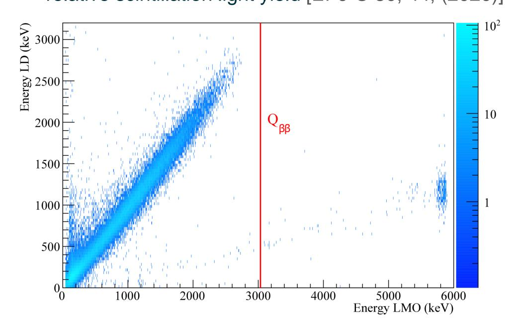
Example of  $\alpha$  discrimination for a detector after 200 days of physics data from March 2019 – April 2020; the LD is cross-calibrated against the  $\text{Li}_2\text{MoO}_4$  energy scale for  $\beta/\gamma$ events.  $\alpha$ 's emit only ~20% of light, compared to  $\beta/\gamma$ .
