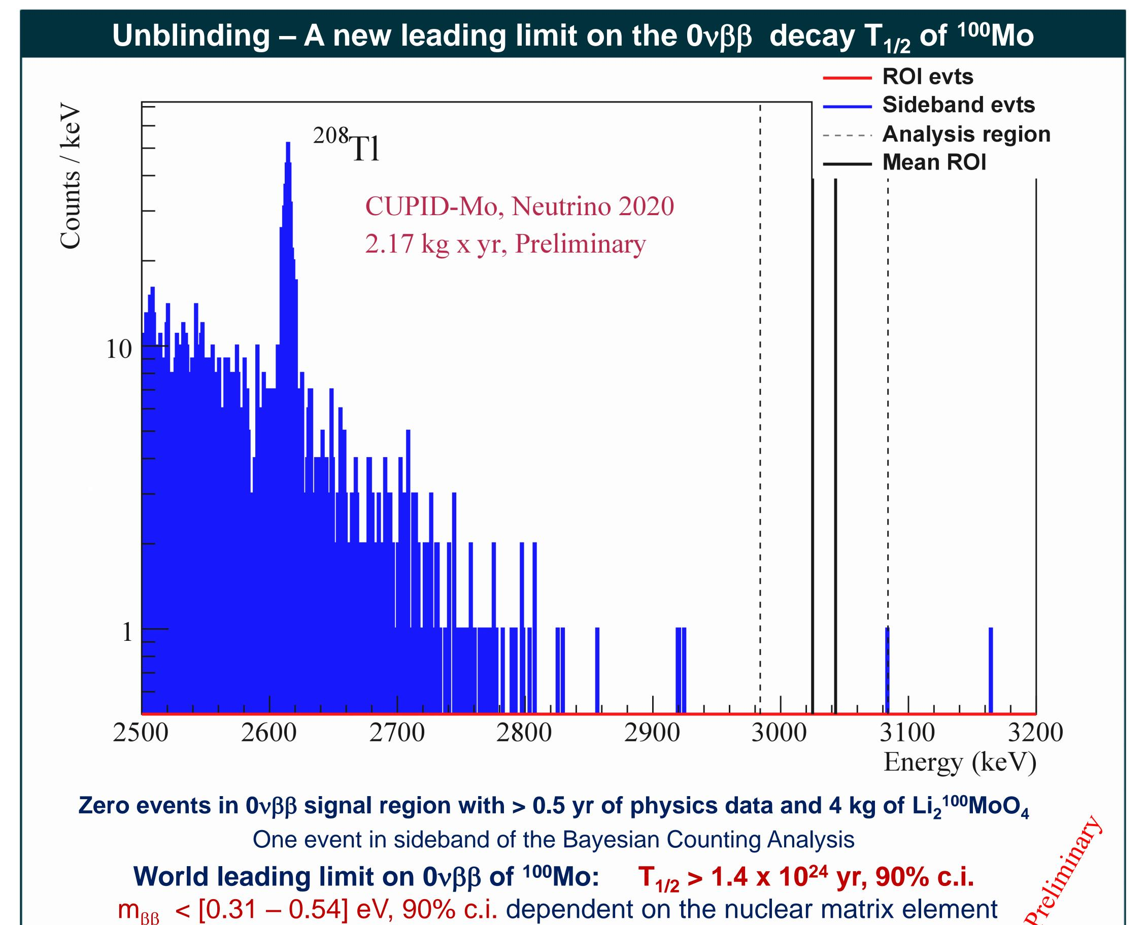
Important step in demonstration of the detector technology for CUPID
