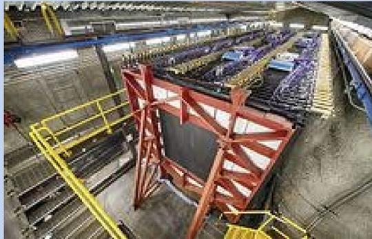
The detectors are made from PVC extrusions which segment the volume in to 4x6 cm cells which alternate orientations to provide 3D tracking of particles in the detector.
