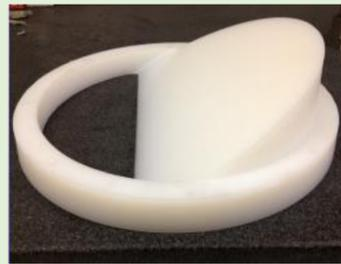
In Emittance Exchange a muon beam is passed through a dipole magnet to create both a position spread and a position-energy correlation in the beam. The beam is then passed through a wedge of specific thickness to eliminate the momentum dispersion. The beam then has an increased longitudinal phase-space density and a reduced transverse phase-space density. The emittance has been exchanged. The transverse emittance can then be reduced by ionisation cooling.
