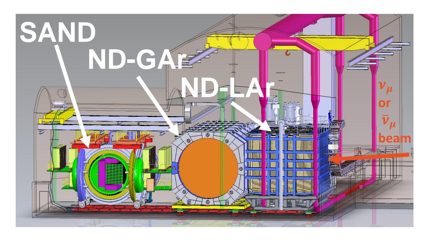
The System for on-Axis Neutrino Detection (SAND) [3] will be part of the DUNE near detector. It is based on a superconducting magnet and an electromagnetic calorimeter (ECAL), repurposed from KLOE (K-Long Experiment) [4].
