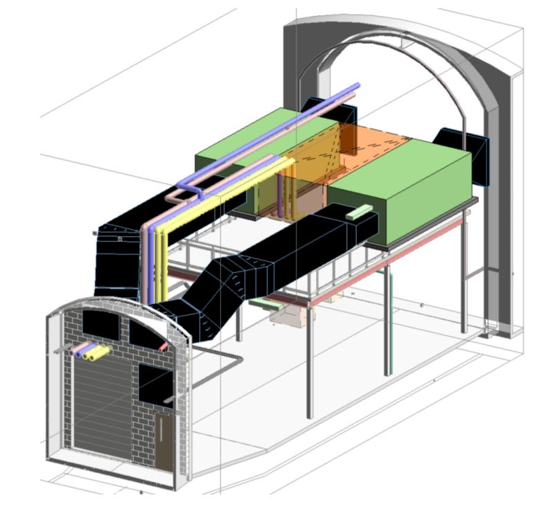
OPTION NOT PREFERRED DUE TO SUPPLY DUCTS EXISTING ON BOTH SIDES OF MONORAIL
