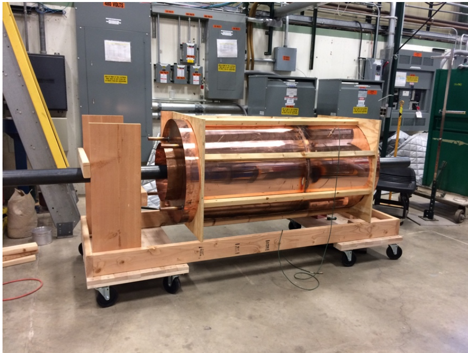
Figure 4.25: Prototype of Recycler 53 MHz Cavity with a \frac{R}{Q} of 45
