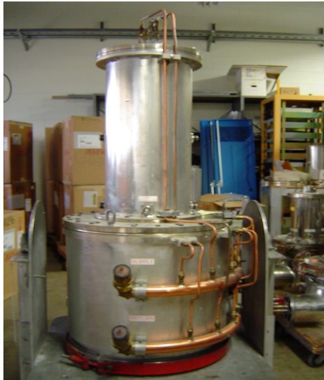
Figure 4.19: Main Injector Power Amplifier, Eimac Y-567B Power Tetrode
