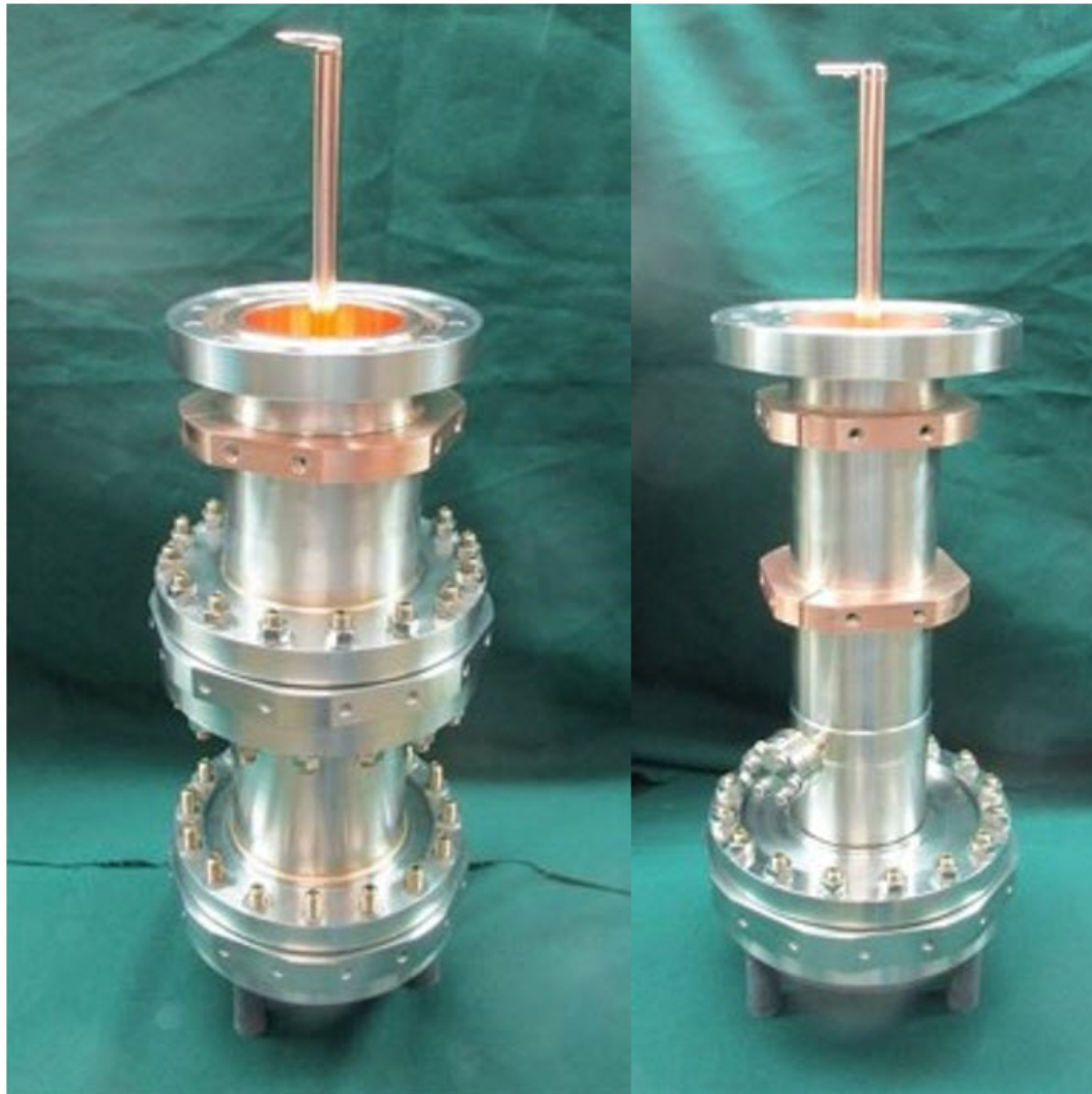
Figure 7.63: Vacuum parts of couplers with electromagnetic shields. No copper coating on left and with copper coating on right.
