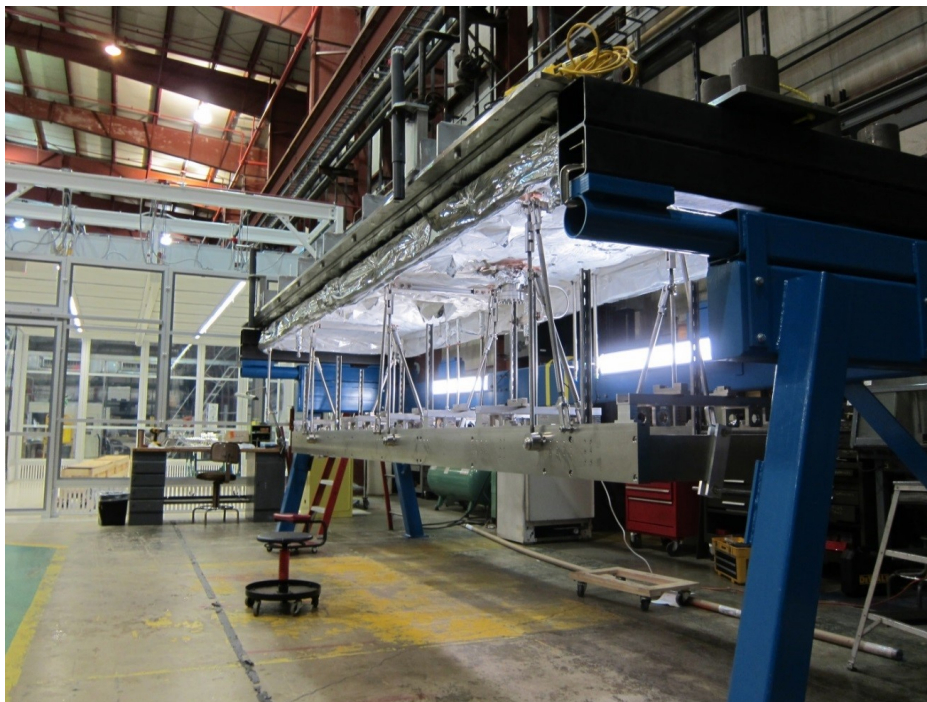
Figure 7.14: The titanium strong-back hung from the lid of the half-wave resonator lid. No cavities or solenoids are mounted on the strong-back.
