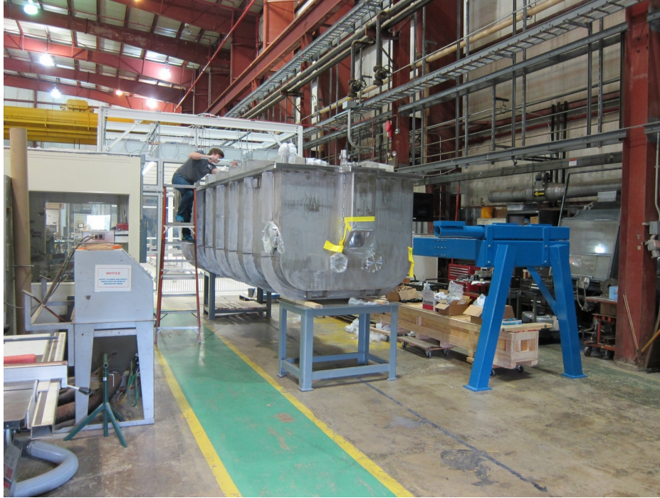
Figure 7.13: The finished vessel assembled at Argonne. The vessel is now being prepared for cryogenic testing.
