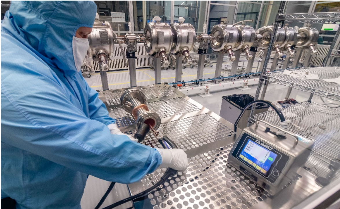
Picture 6: Counting of particles coming from assembly.
