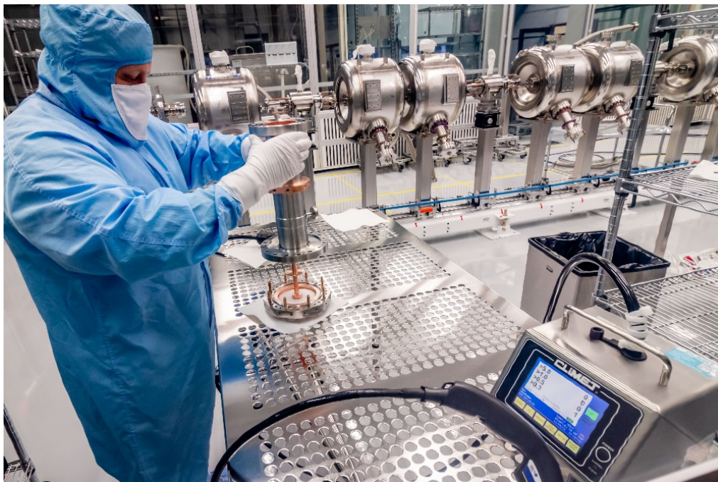
Picture 5: Assembling of outer conductor with antenna.
