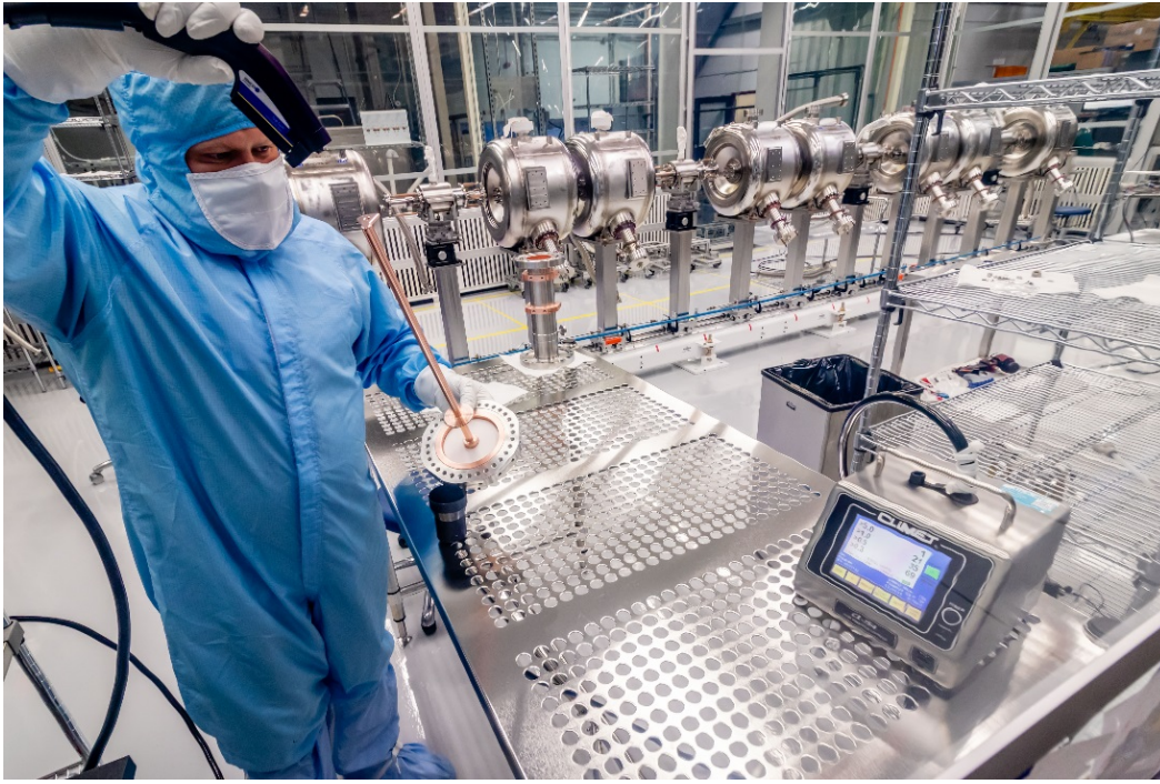
Picture 4: Cleaning of antenna with Nitrogen gun.
