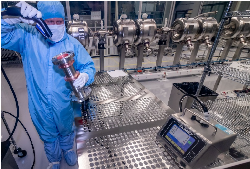
Pictures 3a and 3b: Cleaning of outer conductor with Nitrogen gun.
