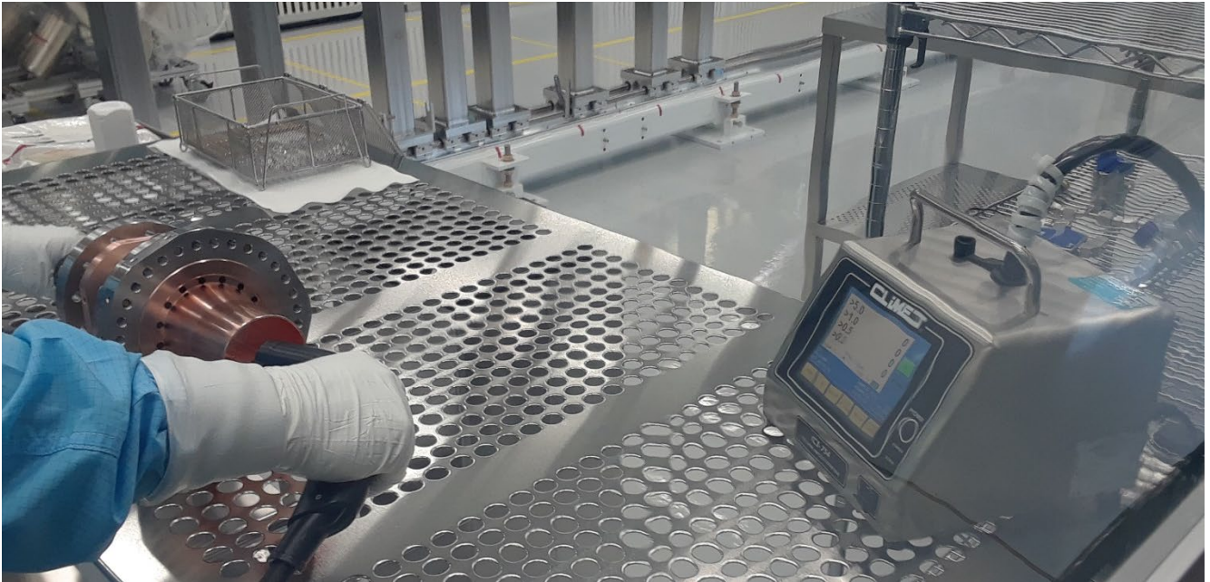
Picture 4: Intermediate test for particles. Zero number of particles on the counter screen.
