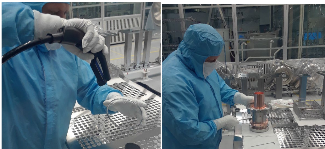
Picture 3: Clearing parts by flow of Nitrogen before assembling and assembling.
