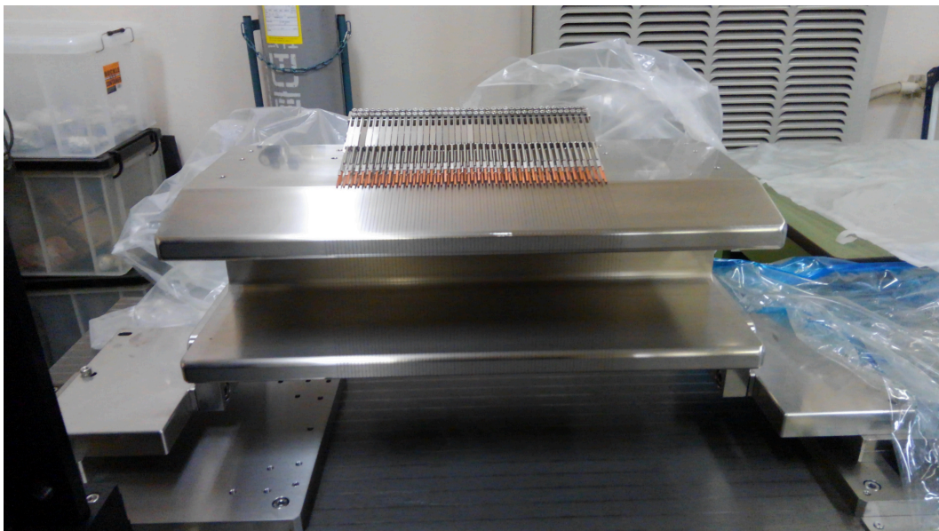
50cm yoke to strain CNT wires ( \phi 150 \mu\text{m} CF wires)
