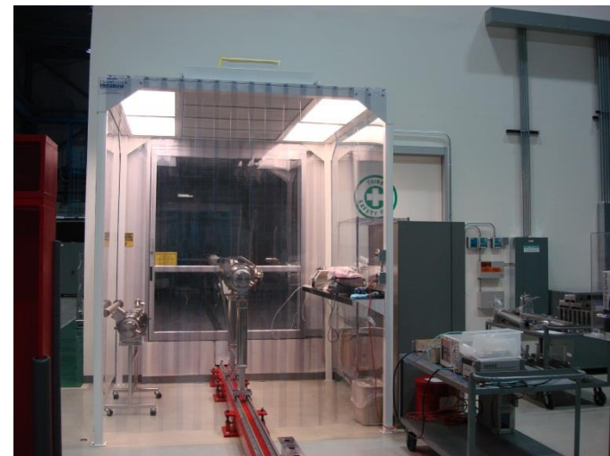
Class 1000 softwall cleanroom for dry cleaning before entry to ante cleanroom
