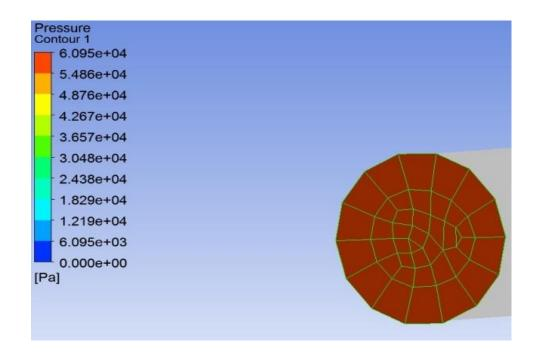
Pressure Drop is 3.654 bar @ velocity 2.5 m/s, diameter of coil is 6 meter, dia is 20mm
