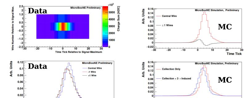
Average signal shape reconstructed by lining up signals in time; include central and side wires
