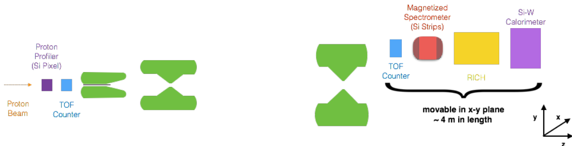
Figure 2: Sketch of LBNF target/horn system and one possible LBNF spectrometer design. Not to scale.
