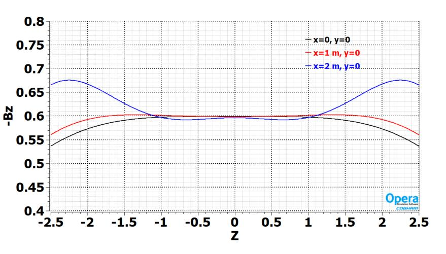
The center field is 0.6 T at coil total currents: 0.98 MA (center and shield), 2.44 MA (side).
