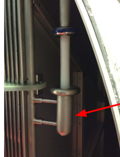
HV connection at the Cathode cup inside the cryostat
