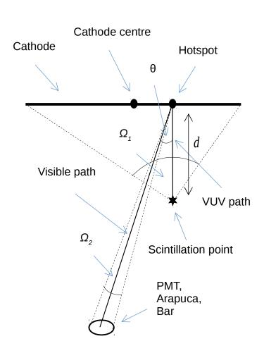
Semi-analytic model for visible light from TPB coated foils on the cathode:
