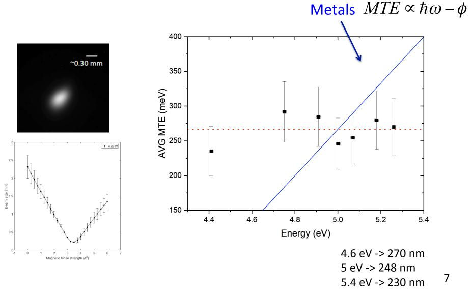
Is MTE due to one-step photoemission from low effective mass graphitic boundaries? Change the sp3/sp2 ratio (how much graphite) and look at MTE
