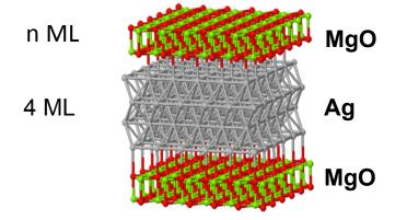
The number, n, of ML controls the location In k-space where the valence band crosses the Fermi level
