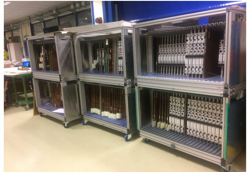
A photograph taken in December 2018 showing some of the large size GE1/1 chambers that have been constructed and stored in racks at CERN Prevezsin building 904.
